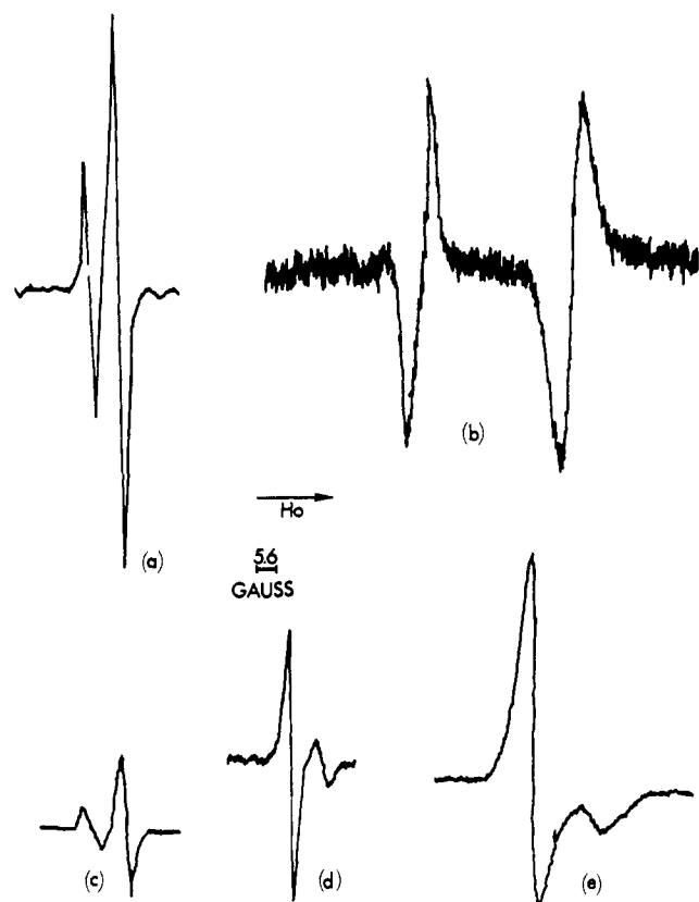
Figure 1. ESR spectra of the chromium(V) intermediate in the chromic acid oxidation of oxalic acid: (a) 50% AcOH; (b) 50% AcOH in Q-band; (c) water; (d) 100% AcOH; (e) 50% AcOH at liquid nitrogen temperature. All measurements except b are in X-band; all measurements except e are at 25°. Concentrations: (d) \text{CrO}_3 = 0.00042 \text{ M} , oxalic acid = 0.019 \text{ M} . All others: \text{CrO}_3 = 0.00081 \text{ M} , oxalic acid = 0.076 \text{ M} , \text{HClO}_4 = 0.024 \text{ M} .
